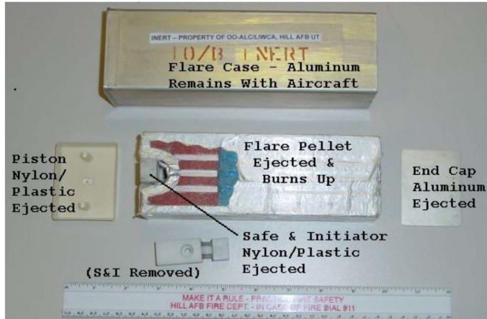
Figure 7-8. MJU-10/B Flare with Aluminum Case Cut Away to Show the Different Materials
