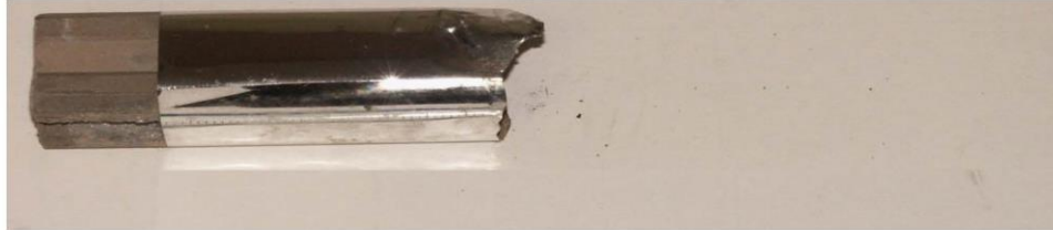
Figure 7-29. Approximately 40 Percent of an M-206 Dud Flare
