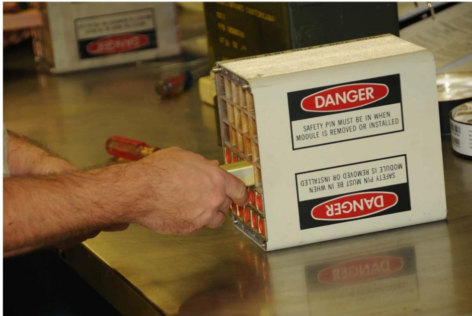
Figure 7-7. A Flare Magazine that Holds Thirty 1-inch by 1-inch by 8-inch Flares
